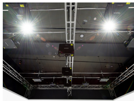
Panasonic DLP Laser projectors with ultra short throw lenses rigged on the ceiling enabled ACMI to create immersive experiences for their visitors.
